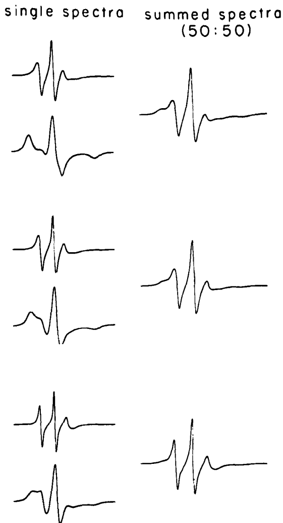
FIG. 9. The effect of line shape changes in individual components on the final composite ESR spectrum. Left column: The pairs of spectra are scaled arbitrarily to the same center line height. The upper spectrum of each pair is characteristic of the 14-proxylphosphatidylcholine in lipid bilayers. The bottom spectrum of each pair shows the line shapes of the broad protein-associated components. The changes in these individual line shapes, from top to bottom, are characteristically seen with increasing temperature, as the bilayer lines narrow and the outermost features of the broad component decrease slightly. Right column: The summed spectra were obtained by integrating and summing, so that two components on the left are present in equal amounts. The change in line shape from top to bottom mimics the line shape changes that occur with increasing temperature. Note that both components remain present in the same ratio, despite the radical changes in appearance.
